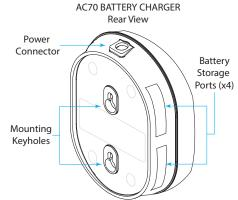
Note: Storage Ports do not charge batteries Fig. 2
